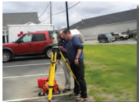
Deputies being trained on the "Total Station" for Forensic Mapping.
